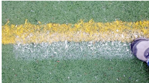
Excessively Worn Fibers with Shedding
